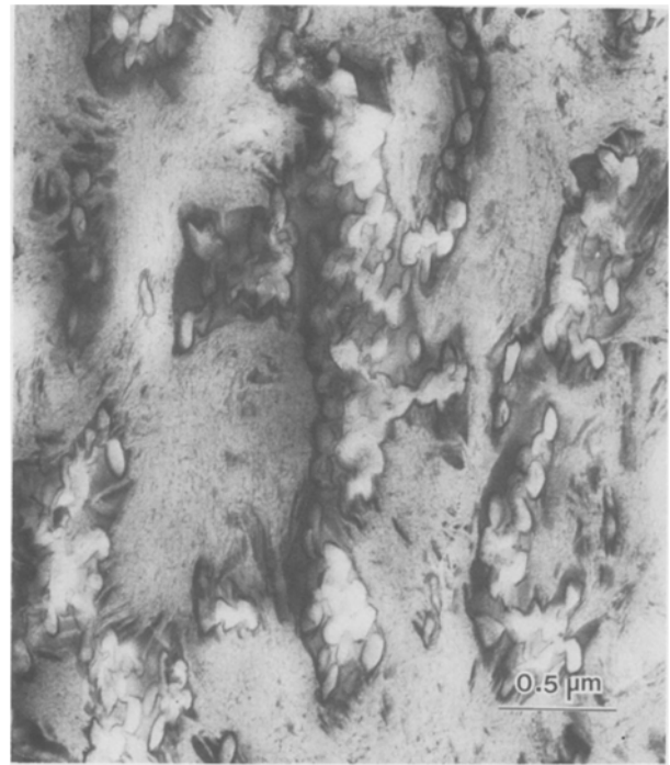
Figure 10 Transmission electron micrograph of thin section of recrystallized Blend 3 showing detailed morphology of PBT and PC phases separated during slow cooling.
